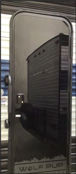
Real Blackout Glass, Safety Slam, Friction Hinge Entry Door with Window and Shade Prep
