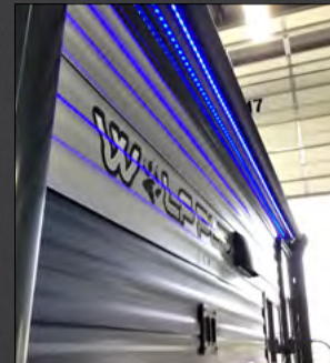
Exterior LED Light Strip at Awning
