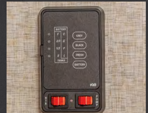
Monitor Panel for Tanks and Battery Levels
