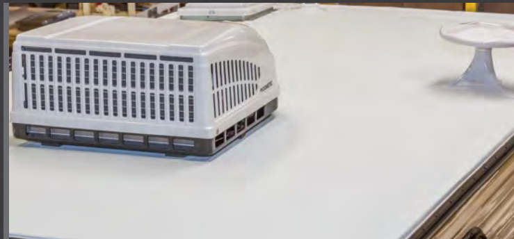
One-piece, Walkable Decked Roof
