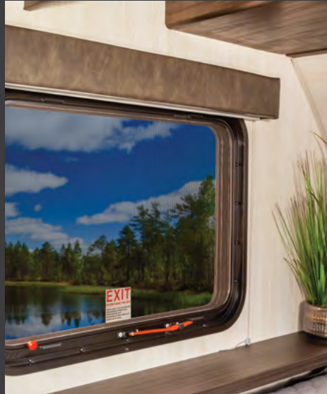
Emergency Exit Windows
