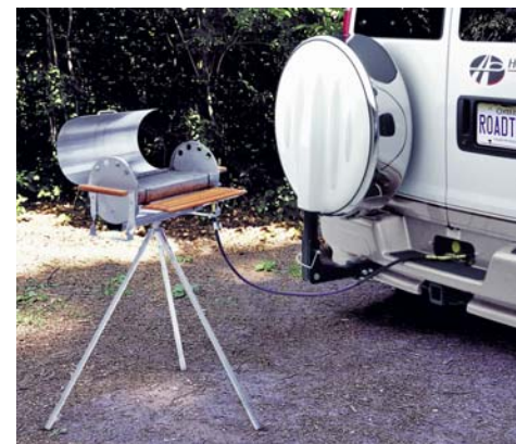
External propane barbecue connection with quick disconnect.
