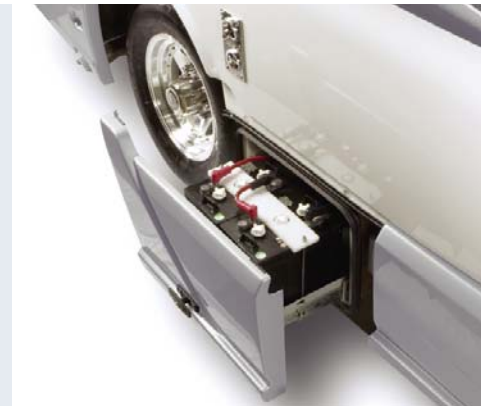
210 and Sprinter based models feature an optional auxiliary battery system with two lead acid deep cycle 6V batteries with 220 total amp hours located in a convenient slide-out drawer.
