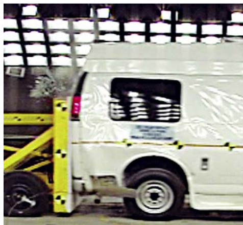
This photo shows the rear impact test. The test vehicle was impacted by a moving barrier at 30-mph (48 km/h). The entire fuel system was then inspected for leakage. Our test vehicle did not leak any fuel.
