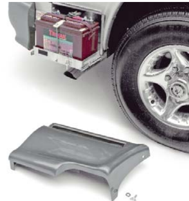
A large capacity auxiliary lead acid battery is totally concealed yet easily accessible on slide-out tray. A second auxiliary battery is optional on all models except the 170.
