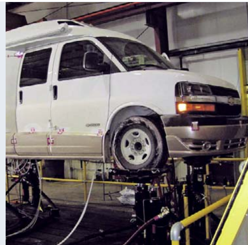
"Automotive manufacturer" style durability testing allowed us to quickly identify and implement numerous design improvements which would otherwise only become apparent during the normal life of the first vehicles built and sold.
