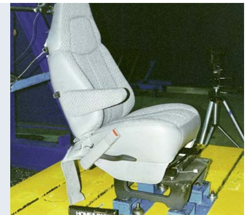
Seating system testing minimizes the possibility of failure of the seats, their attachments and their installation.
