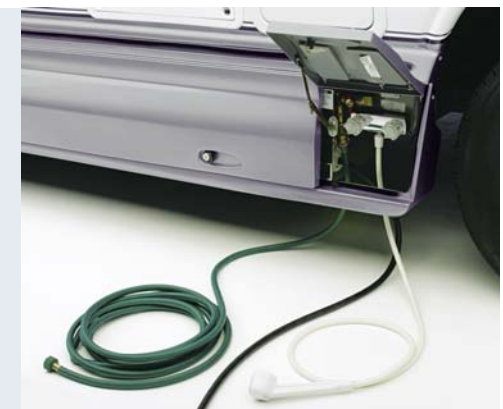
There is a separate compartment for an exterior shower and city water connection with quick disconnect. The 210 and SS feature a detachable power cord for trips away from the campsite.
