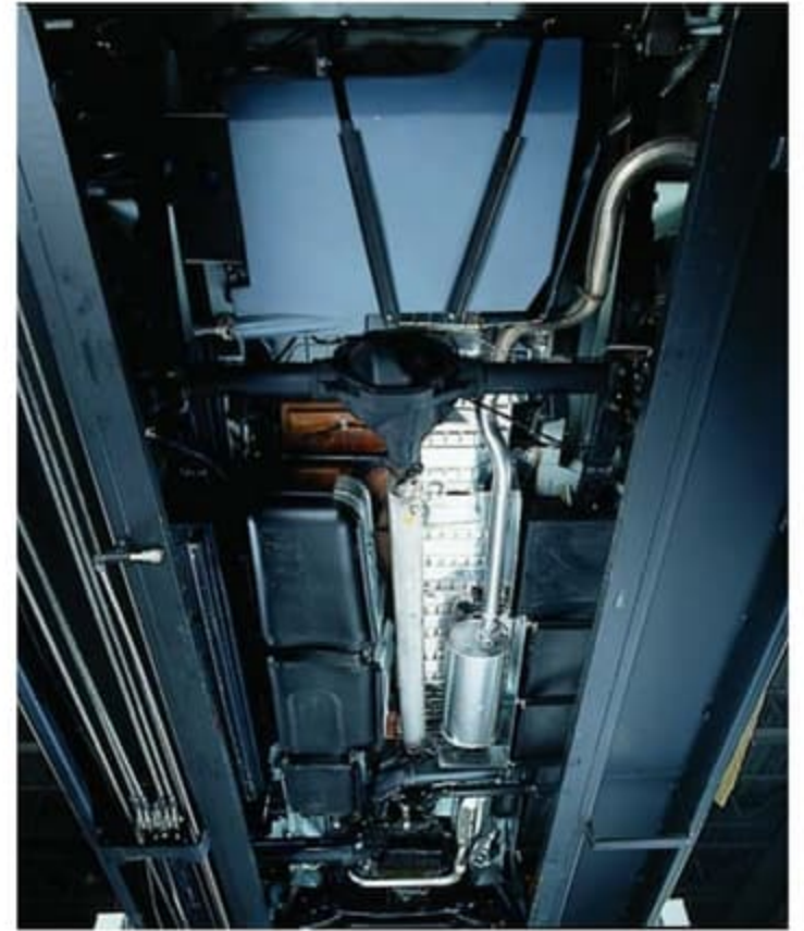
Water tanks fit below the floor to maximize interior storage space and improve weight distribution for better handling.
