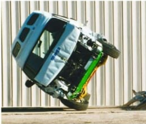
Dynamic rollover testing is intended to reduce deaths and injuries from occupants and their appendages not remaining within the passenger compartment during rollover accidents.
