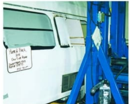
These photos depict side crush resistance testing which is intended to simulate the vehicle impacting a utility pole at a perpendicular angle.
