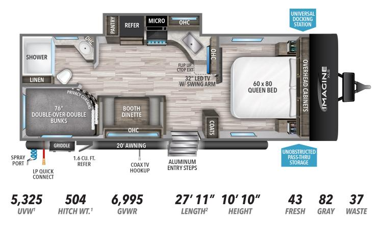
1 Based on average weight in lbs. 2 Hitch to rear. Water Capacities in Gallons.
