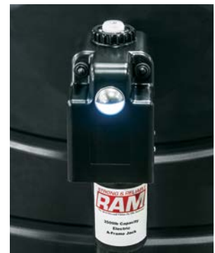
The power tongue jack (TT shown) is included in the Touring Package or as a separate option.
