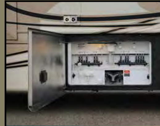
BERKSHIRE XL'S WATER MANIFOLD SYSTEM WITH WHOLE UNIT FILTER AND EXTERIOR SHOWER
