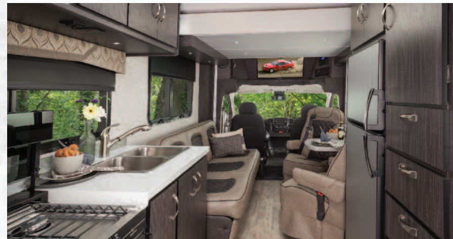
The well appointed galley has a three burner stove top, a seven cu. ft. refrigerator, a solid surface countertop, a tankless hot water heater and plenty of storage.
