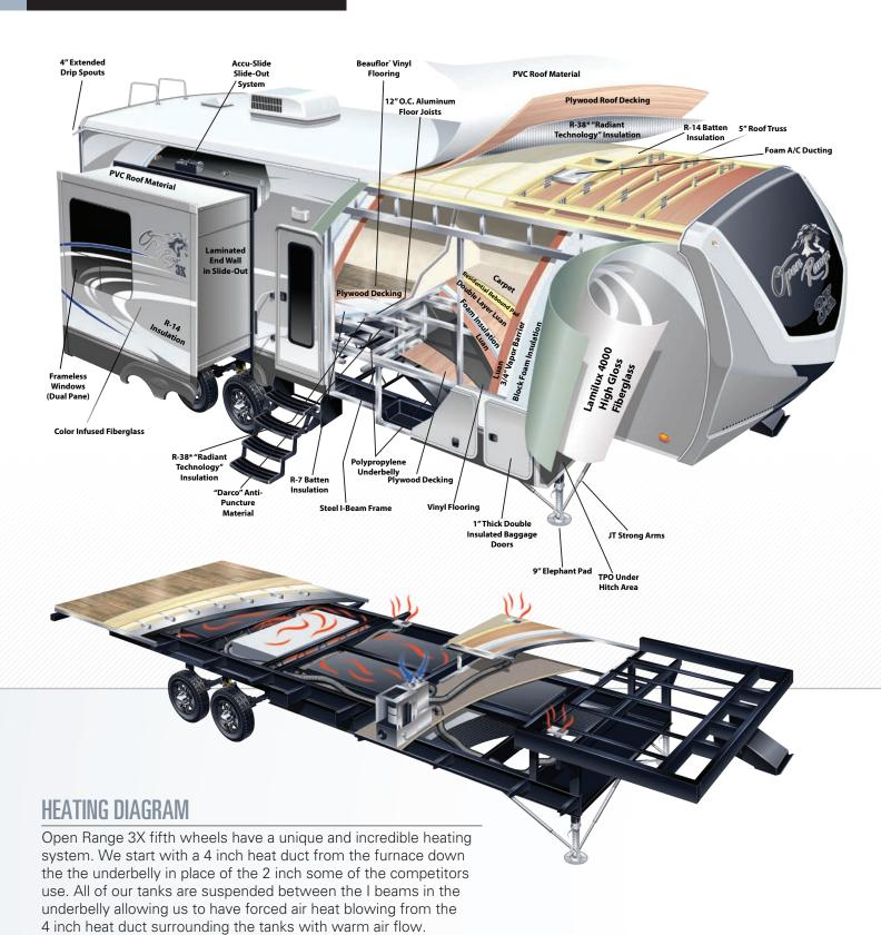
How do we get the air flow? Simply by having a return at the end of the tanks going back into the coach. The secret is that simple. We put a return in their underbelly to allow air flow over the tanks instead of a pressurizing system that occurs in other brands.
