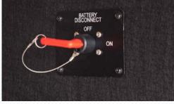
Battery Disconnect in Pass-Thru Storage Area
