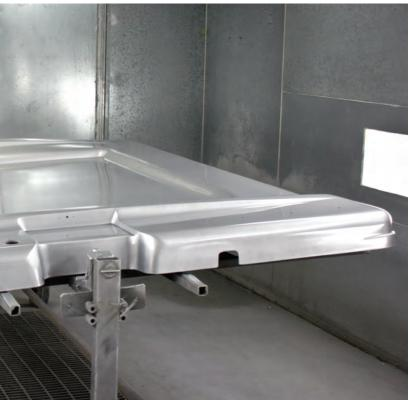
integrity of that piece. After the fibreglass has been sprayed into the mold, a trained team will methodically hand roll the entire part to ensure that there are no air pockets and the fibreglass is uniform throughout the part. This time-consuming process further ensures that each component meets or exceeds our high quality standards.
