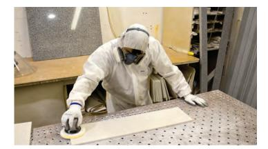
polishing to achieve the beautifully deep and rich seamless solid surface look that conforms to our exacting standards. This is an extremely labour intensive process. On average, we spend a total of sixteen hours hand-sanding and polishing the Corian<sup>®</sup> surfaces in our motorhomes.
