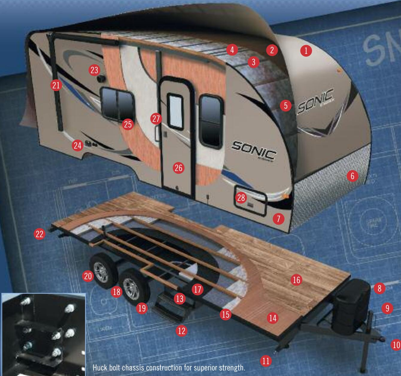
1. One-piece fiberglass roof from front profile to rear bumper
