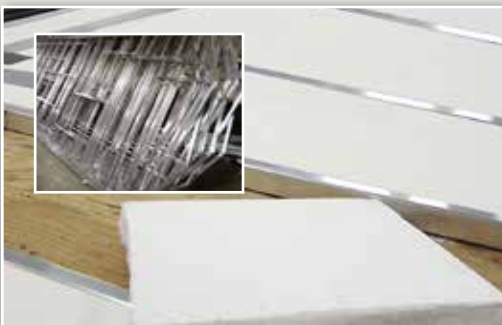
Laminated Sidewall Construction
