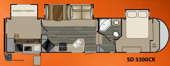
Length: 36' 10" Height: 12' 4" Dry: 10,700 GVWR: 13,920 Hitch: 2,165 Tanks: 53<sup>F</sup> 80<sup>G</sup> 40<sup>B</sup>
