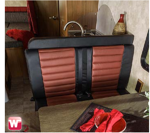
The dinette bench seat in the Trend is the first in the industry to come equipped with 3-Point Seat Belts .
