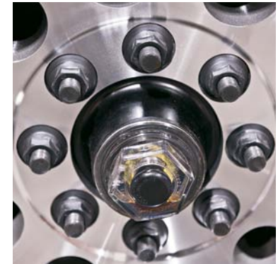
Commercial oil bath hubs surrounded by 8 large 5/8" stud bolts and standard automotive disc brakes round out the safety features of every DRV unit.
