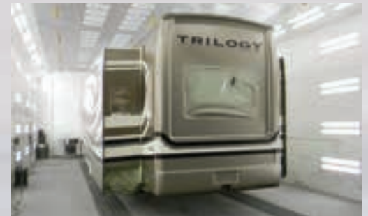
Three coats of clear top the base coat colors and logos. Next, the unit is baked for one hour at over 150°. After sanding, an additional three coats of clear are applied and baked for an outstanding finish.
