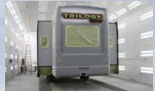
Logos are applied with the use of digitally plotted spray masks.
