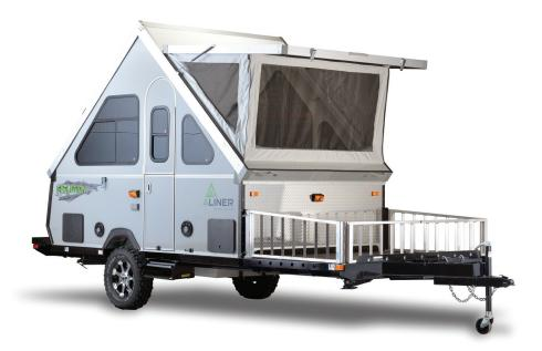
The **Evolution**, based on the larger chassis of its best-selling sister company, Somerset — meets the demands of extended stays off the grid. It offers a 35-gallon water tank, LED lighting, and versatile front and rear decks to carry everything from camp chairs, gas cans and toolboxes to coolers, firewood and bicycles. Even a quadl Lightweight, heavy-duty alumn
