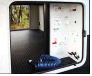
The newly updated fully enclosed and LED lighted docking center includes a removable coiled hose outside shower, black tank flush, winterization kit, water heater bypass, battery disconnect, and dedicated cable and satellite jacks.
