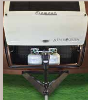
(left) Aerodynamic lines are preserved with the front panel closed (right) Storage in the front panel for two LP tanks and dual batteries
