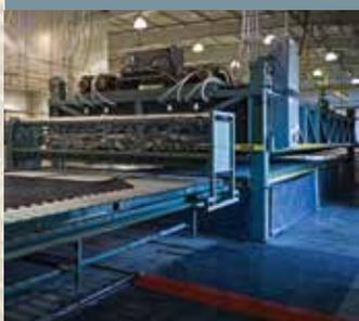
Ever-Lite is built with vacuum lamination in the walls, roof and floor. Dense, block foam insulation is coated with a water-based urethane adhesive which becomes super bonded under the heat and high pressure of EverGreen's vacuum lamination process. The result is a stronger, yet lighter and more durable coach that's better insulated for all seasons.
