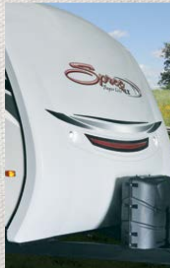
Aerodynamic one piece front end cap with integrated LED lights.
