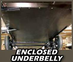
Eliminates turbulence caused by exposed frame members, holding tanks,plumbing etc.
