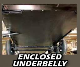
Eliminates turbulence caused by exposed frame members, holding tanks, plumbing etc.
