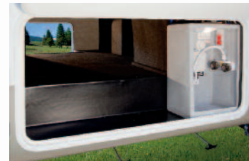
Pass thru storage with docking station
