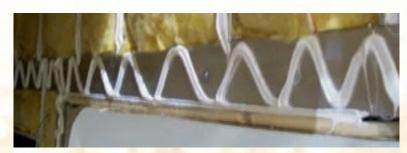
Thick Silaprene (475 PSI) guarantees solid contact between the gelcoat and aluminum frame without lamination
