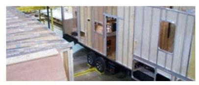
Aluminum studded sidewalls and roof trusses on 16" centers or less
