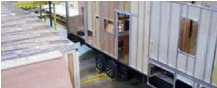
Aluminum studded sidewalls and roof trusses on 16" centers or less
