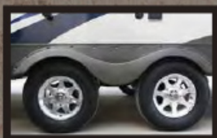
WIDE TRACK SUSPENSION (TRAVEL TRAILERS ONLY) WITH ALUMINUM RIMS
