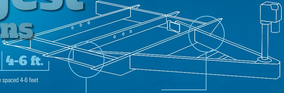
**Eagle travel trailer integrated A-frame:** The A-frame runs through the main frame, preventing the hitch from buckling like competing tack-welded frames.
