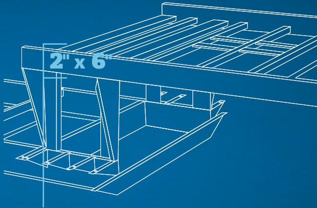
**Fifth wheel frame:** The frame over the truck bed is built on a superior 2" x 6" tube perimeter structure to better support the bedroom sidewalls. Competing fifth wheels have a smaller frame; these manufacturers add a sidewall support seam to compensate for expansion joints.
