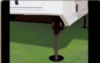
Hydraulic Front Landing Gear Are Fast And Powerful (6 point Auto Leveling is optional)
