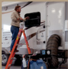
Seal Tech Air Pressure Test
