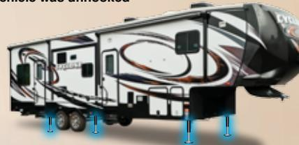
• Utilizing a remote sensor located under the rear axle, the Level Up system accomplishes a level coach in seconds. This eliminates a time consuming and sometimes dirty task of manually leveling your coach.
