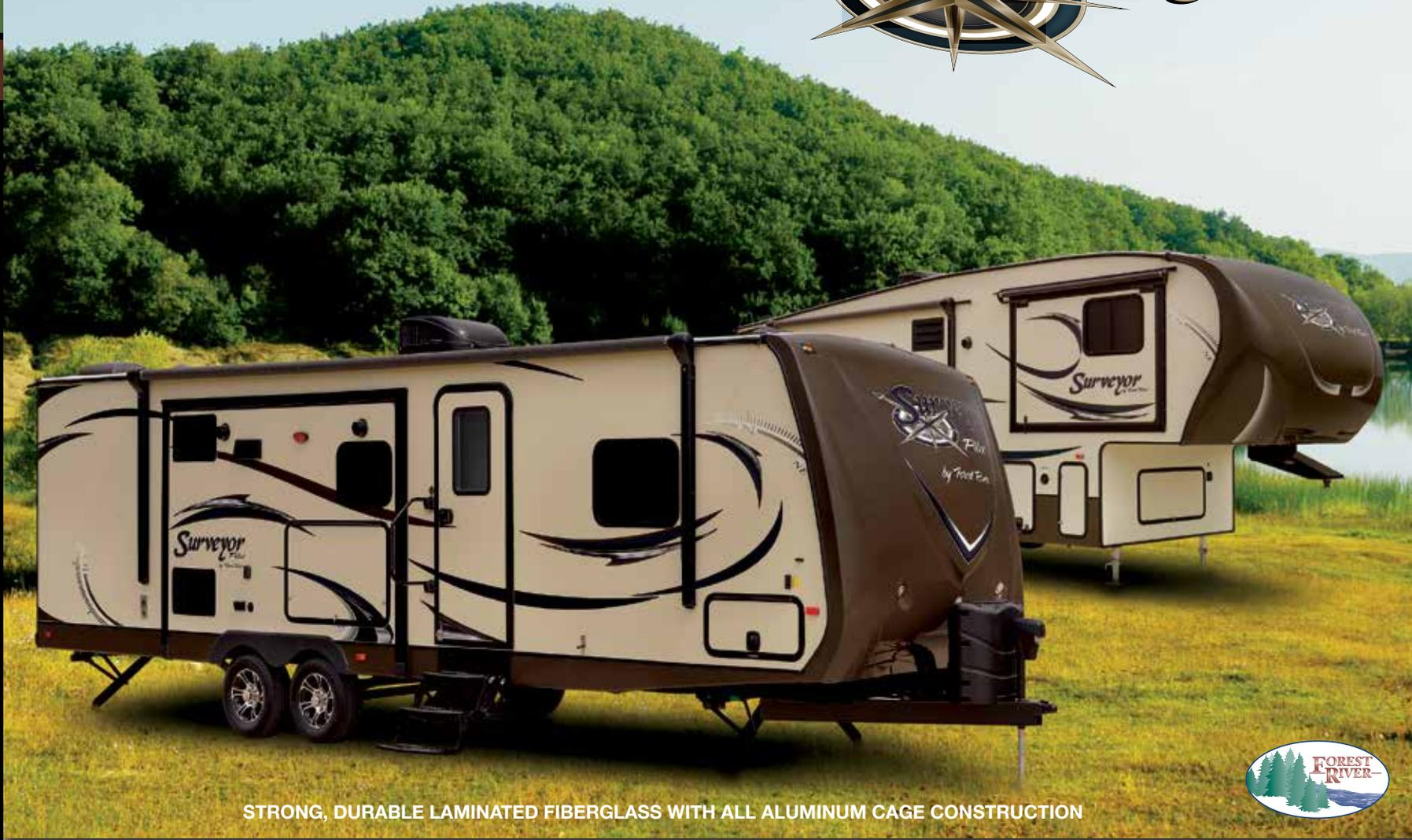
**STRONG, DURABLE LAMINATED FIBERGLASS WITH ALL ALUMINUM CAGE CONSTRUCTION**
