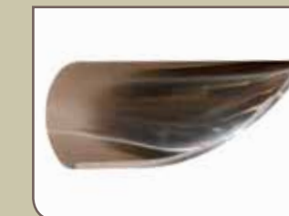
Nose cone w/protective keel. Industry standard has 48" nose cone. Berkshire has engineered a longer 52" nose cone to enhance speed, reduce gas consumption & provide a more comfortable ride.
