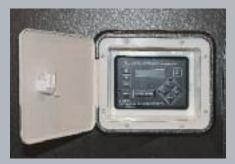
This electronic leveling control panel provides a one-touch auto-level feature. When it's time to depart, auto re-hitch memory restores the coach to the unhooked position. To retract, scroll to auto retract, press "enter" and in 20 seconds you're ready to hit the road.
