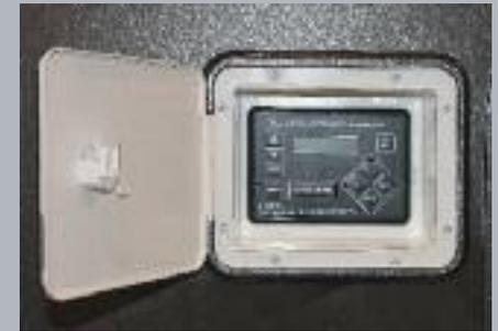
This electronic leveling control panel provides a one-touch auto-level feature. When it's time to depart, auto re-hitch memory restores the coach to the unhooked position. To retract, scroll to auto retract, press "enter" and in 20 seconds you're ready to hit the road.
