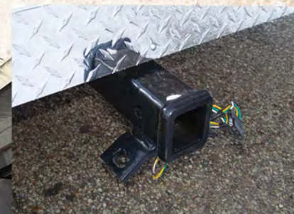
Rear mount 2" hitch receiver for small trailer or bumper gear rack.
