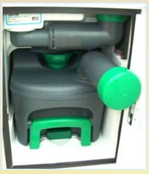
With the exterior door open you simply lift the green lever and slide the 5.1 gallon black tank out. Top tube is the fresh water fill that also swivels out to fill easily.
