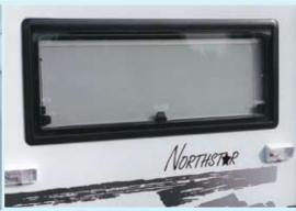
The screen rolls down from the top and the shade up from the bottom. They can be quickly and easily connected so you can position them how you would like. When the shades are up you have total privacy. Quickly roll your screen or shad back and enjoy an unobstructed view. Open the window to pass items in and out of the unit.
