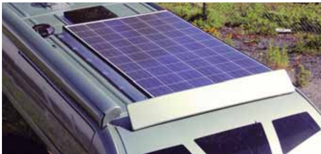
240 W solar charging system provides power as long as there is daylight - not just sunshine.
