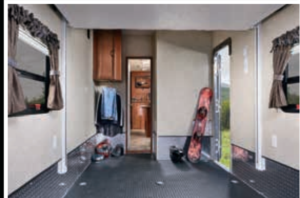
359THKS The 12' garage includes heavy duty tie-downs, anchored into an 8" x14" steel plate welded to the frame for secure travel. Optional dual electric queen bunk beds add cargo area sleeping quarters. A fuel station option is available.
