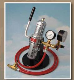
A pressurized LP line test ensures that your unit is safe and all LP gas components are in working order.
