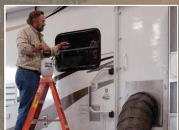
When checking for water leaks we pressurize the unit and then use a Seal-Tech spray on every part of the unit to identify any problem areas.
