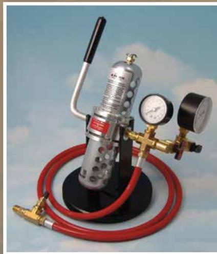
*A pressurized LP line test ensures that your unit is safe and all LP gas components are in working order.*
