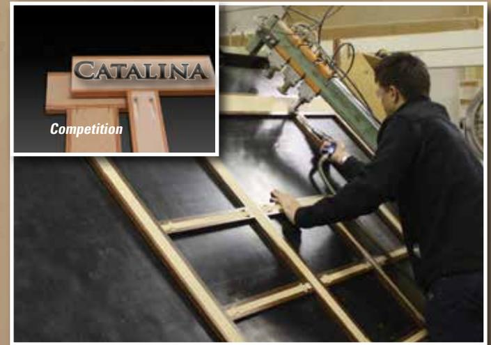
*All of our craftsman are thoroughly trained to use a framing table with jigs and clamps. This ensures that the cabinets are built to extremely tight tolerances for tight and secure cabinetry that will last for years.*
