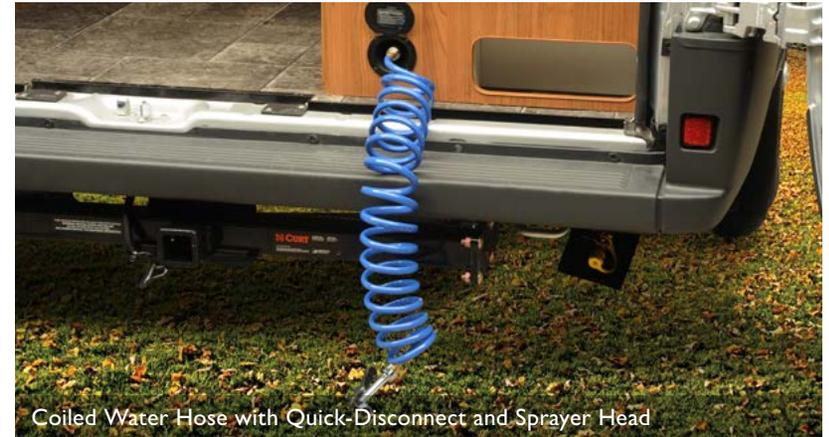
Coiled Water Hose with Quick-Disconnect and Sprayer Head
