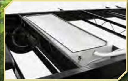
HEATED AND ENCLOSED FRESH WATER TANK
