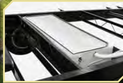
HEATED AND ENCLOSED FRESH WATER TANK
