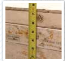
7" HEADER BEAM VS. 2" X 6" LUMBER
