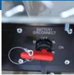
12 Volt Disconnect provides for easy power shut-off
