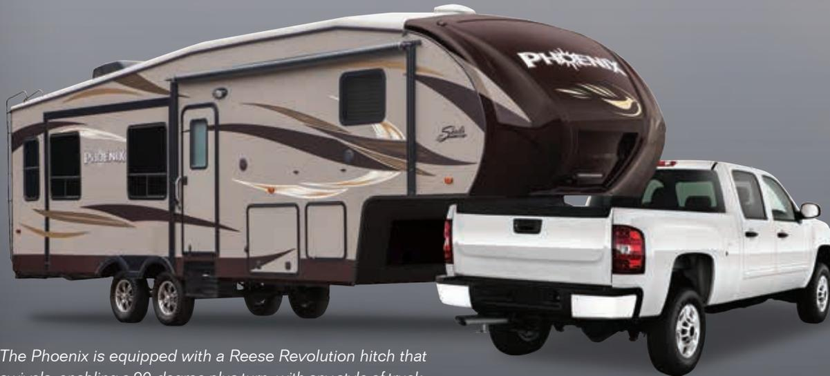
The Phoenix is equipped with a Reese Revolution hitch that swivels, enabling a 90-degree plus turn, with any style of truck.
