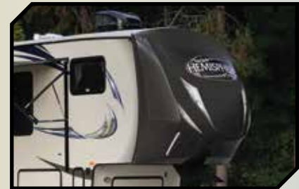
PAINTED GEL COAT FIBERGLASS FRONT CAP ON TRAVEL TRAILERS AND FIFTH WHEELS WITH LIGHT STRIPS. WON'T FADE, CHALK OR CRACK
