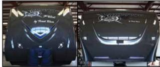
ONE PIECE PAINTED FIBERGLASS FRONT CAPS Surveyor's one piece painted fiberglass front caps provide superior aerodynamics to help save fuel and protect from road debris. Our convenient LED docking lights help you light up when hooking or unhooking at night.
