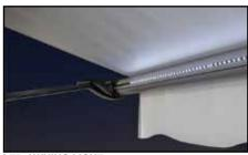
LED AWNING LIGHT The integrated LED awning light provides you with an abundance of light for added safety and security. (Standard in Exterior Luxury package)
