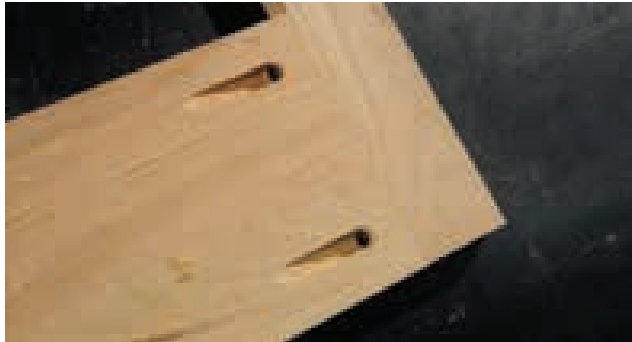
Pocket screws for structural integrity
