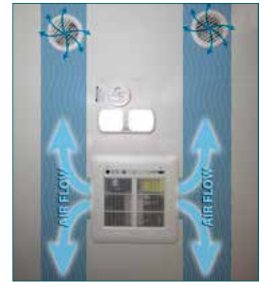
The H-ducted A/C distributes the cool air evenly throughout the travel trailer.
