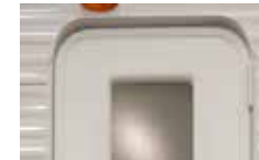
Radius door corners are stronger, last longer and don't tear awnings.
