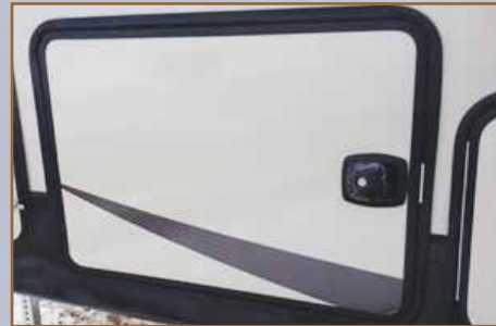
The bus-style slam latch baggage doors provide convenient and secure access to your cargo.
