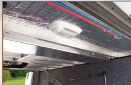
Astro-Foil insulation — insulates under our bed/bath decks and under our slide-out floors.
