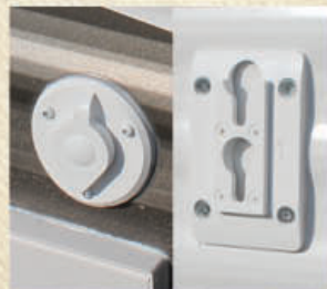
EXTERIOR TV HOOKUP/ CABLE AND BRACKET
