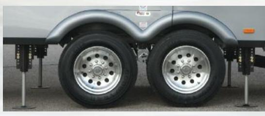
Trilogy is standard equipped with five Goodyear tires. Four are mounted on polished aluminum modular wheels. (Models 3800 RL and 3850 RL have 17.5" H-rated tires; Models 3650 RE and 3650 RL have 16" G-rated tires.)
