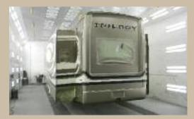
Three coats of clear top the base coat colors and logos. Next, the unit is baked for one hour at over 150°. After sanding, an additional three coats of clear are applied and baked for an outstanding finish.
