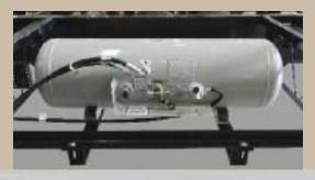
A 97 lb. LP tank is securely mounted between frame rails. Fill and vent valves, are accessed in the docking station. Trilogy is also equipped with a 20 lb. exchangeable auxiliary LP tank.
