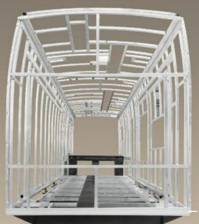
The roof structure is framed with  $1-\frac{1}{2}$ " x  $1-\frac{1}{2}$ " .062 gauge aluminum tubing and  $1-\frac{1}{2}$ " x  $1-\frac{1}{2}$ " .055 gauge P-tube. 1" x 1" solid wood is inserted into the P-tube for enhanced rigidity and improved screw retention.
